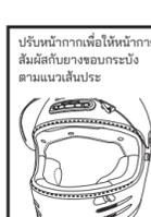
Check point: The upper and lower areas of the inside of the shield/visor should touch the window beading. Adjust so that this part contacts the window beading.
