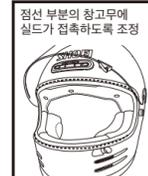
Adjust the shield/visor so it contacts the window beading indicated by the dotted line. Check point: The upper and lower areas of the inside of the shield/visor should touch the window beading. Adjust so that this part contacts the window beading. Cross section of shield/visor. Cross section of window beading.
