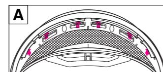
Make it sure that the plate of the front portion of the pad is fixed as shown in diagram A.
