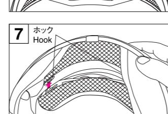
Make it sure that the plate of the front portion of the pad is fixed as shown in diagram A.
