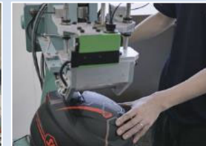
Penetration resistance test
